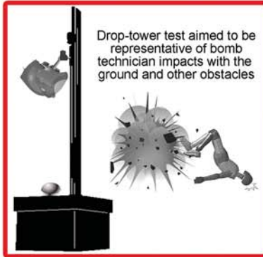
Figure 3: Helmet drop tower testing relevant to traumatic brain injury. 72 drops conducted at 3 temperatures
