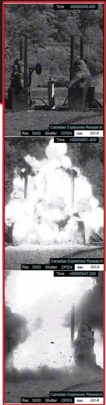
Figure 2: High speed video images of the NIJ 0117.01 blast overpressure test. Kneeling facing 1.25 lbs (0.567 kg) of C4 explosive, at a standoff of 2 feet (0.6 m). Two mannequins used for more data
