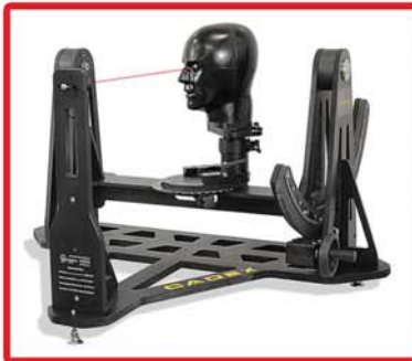
Figure 4: NIJ Static FOV apparatus – helmet fitted on headform and tested at various angles
