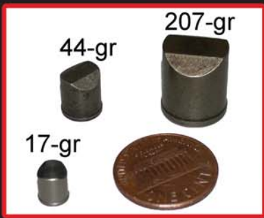
Figure 1: NIJ 0117.01 Fragment Simulating Projectiles (17, 44 and 207-grain)
