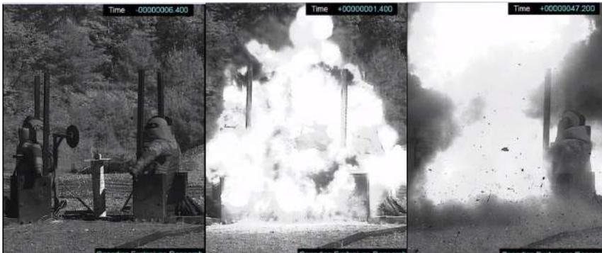
**Figure 3:** High speed video images of the NU 0117.01 blast overpressure test (0.567 kg C4 explosive, standoff 0.6 m - kneeling position). Two mannequins used for more data.
