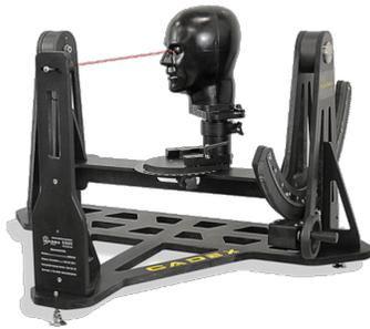
**Figure 4:** NIJ Static FOV apparatus - helmet fitte on headform and tested at various angles
