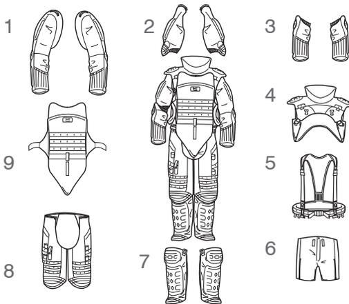
1. Full Sleeve 2. Modular Sleeve - Upper Arm 3. Modular Sleeve - Lower Arm 4. Shoulder Protector 5. Cummerbund/ Suspenders 6. Ballistic Shorts 7. Lower Leg Protectors 8. Thigh Protectors - Front & Rear 9. EOD Plate or Demining Plate (optional)
