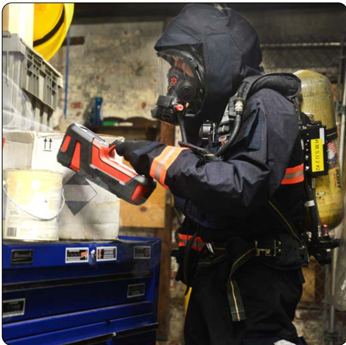
The RedWave XplorIR provides real-time gas and vapor identification.
