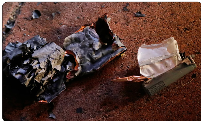
The remnants of an exploded li-ion battery. PETER PEREIRA/ The Standard-Times
